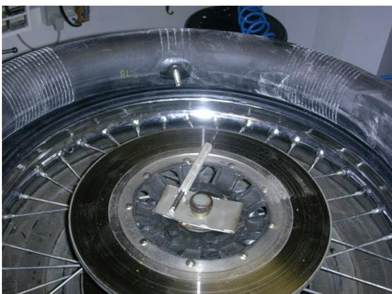
with the tyre removed, it was time to tighten up the spokes, and aligning the rim in both directions. To help in this job, I had build a simple
