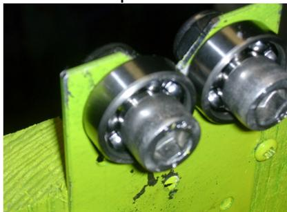
place the wheel at the stand, and rotate the axle a bit. This causes the wheel to start rotating. Let it rest, and mark the bottom position. Repeat – and if the bottom position is the same – place a lead-weight at the spoke pointing upwards.
