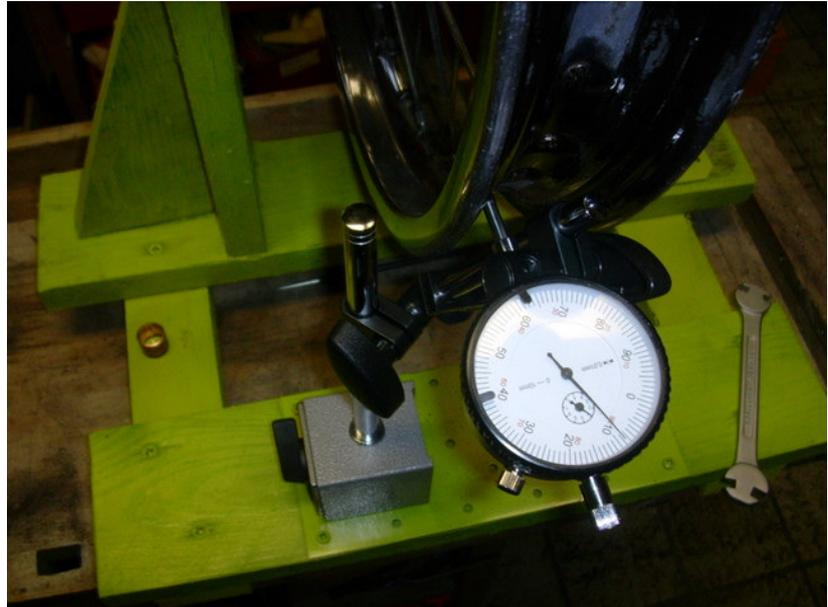
Next job was to get the wheel round. Suzuki says everything within 2mm is o.k. I went for 1/10mm. The principle is to loosen at one side, and tighte at the other to get the round shape.
