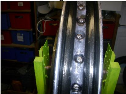
Now it is time to mount the tyre and tube. (Tyres 1<sup>st</sup> side, then put in the tube, and then fix the 2<sup>nd</sup> side) AVOIDING TO HARM THE TUBE.
